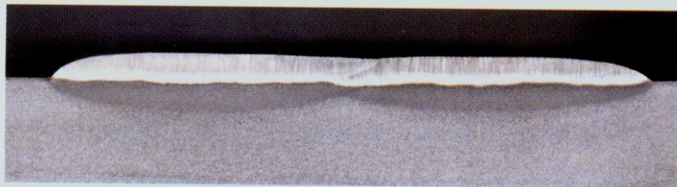
Fig. 11. Cross-section of an Inconel 625-cladding.
